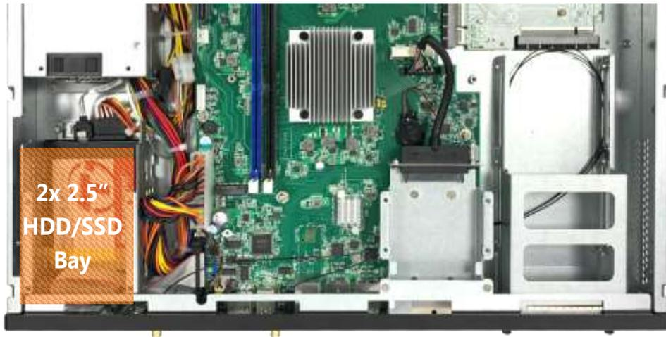
1. Locate the disk drive tray at the corner of the system. Loosen the screw indicated in the picture and slide the tray downwards to have it loosened from the four latching spots. Take the tray out and prepare to install SATA 2.5" disk drives.
