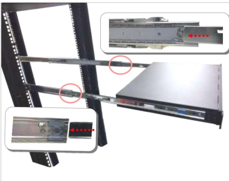
12. While pushing in the system, also push and hold the Rail Lock tab on both brackets.
