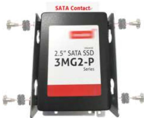
3. Place the tray with HDD/SSD installed back to its original spot inside the system. Remember to aim at the four latching holes. Then slide the tray upwards to get it locked and secure it with the original screw.
