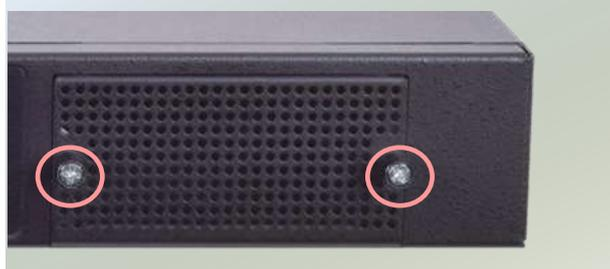
2. Remove the door and locate the PCIe slot for module insertion.
