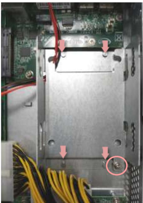
2. Place the disk drive in the tray, as shown in the image below. Apply two disk screws with two rubber washers for each side of the disk drive. If you are going to install two disks, always start by installing the disk in the lower slot.
