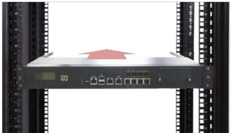
To remove the system from the rack, gently pull it outwards, towards you, while pushing the Release Tab on both sides of the brackets.
