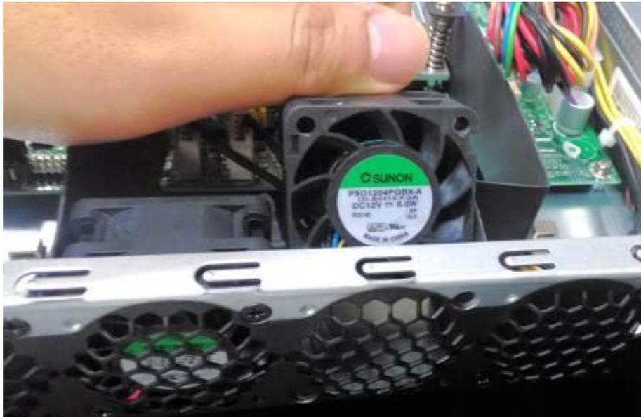
3. To install a new one, just place the new fan to the original place and apply two screws.
