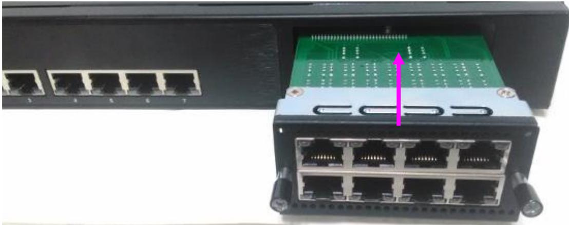
4. Secure the module with two captive screws on the bezel.
