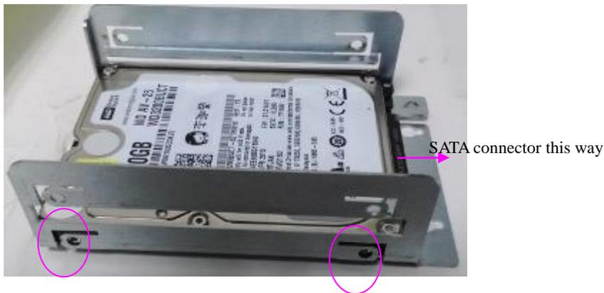
5. Place the tray with HDD/SSD installed back to its original spot inside the system.
