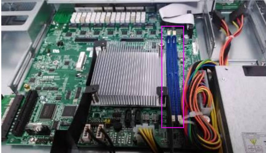
2. Pull open the DIMM slot latches
