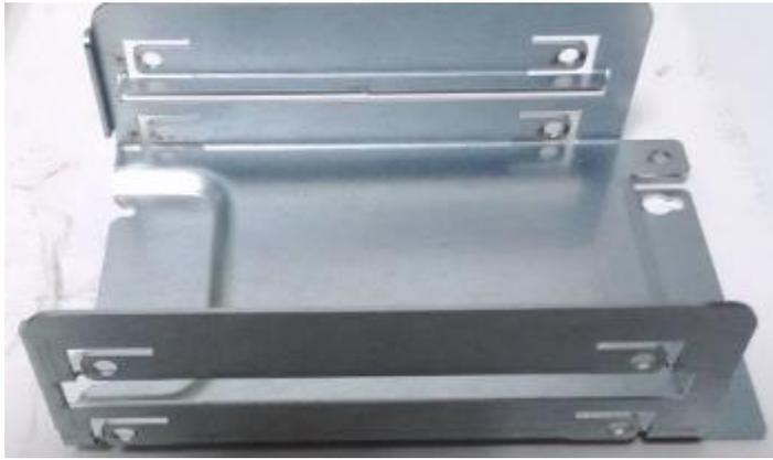
4. Place the disk drive as shown in the image below. Apply 2 screws for each side of the disk drive.
