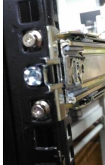
2. For the rear rack installation, also aim at 3 available holes and click the slide-rail assembly onto the rear rack.
