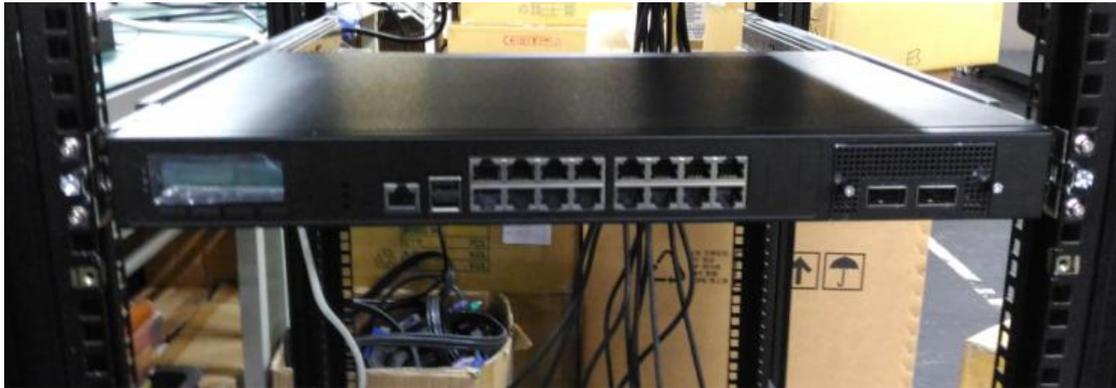
4. To slide the appliance out, gently pull it outwards. Then, press the slide-rail locks on both side and slide the appliance out.
