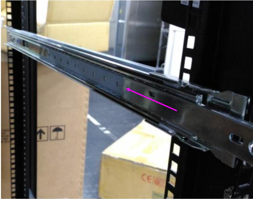
2. Simultaneously push the release tabs on both sides in the arrow of direction below, while pushing the appliance into the end of the rack.
