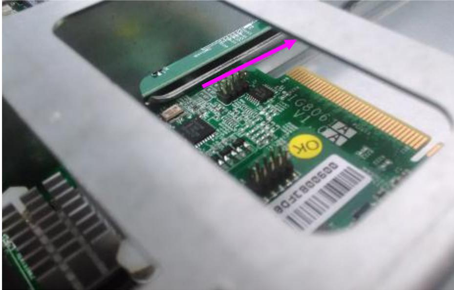
3. Slide your Ethernet NIC module into the space, until it is firmly attached.
