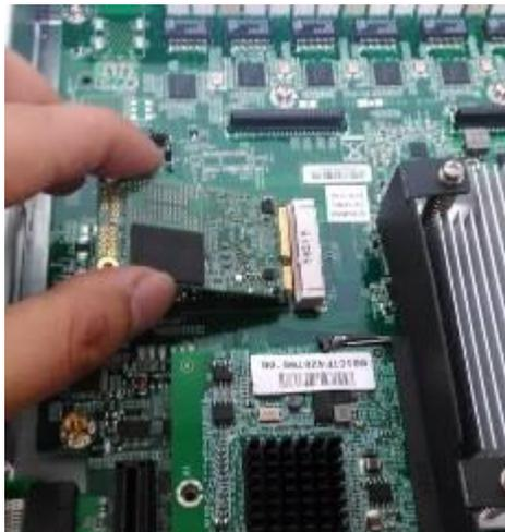
3. Press the module down and apply two screws to secure it.
