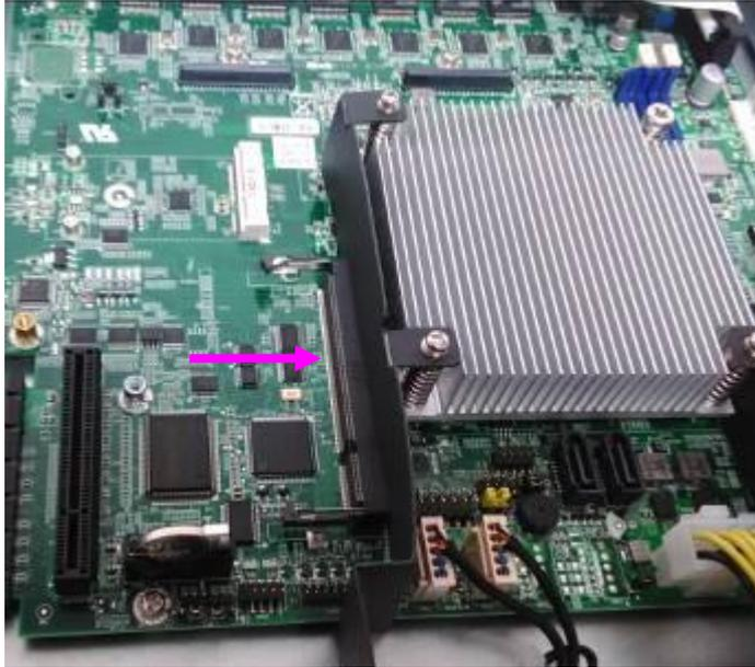
2. Insert an IPMI card into the socket and then press it down.
