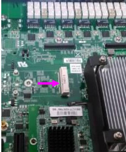
2. Insert a mSATA module as shown in the image below card.
