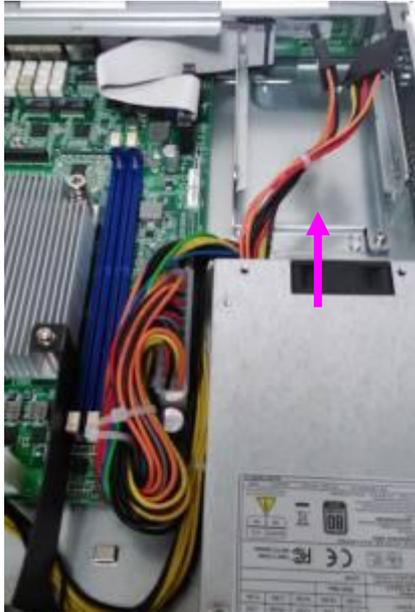
2. Slide the tray downwards. Then the tray will be loosened from the two latching spots.
