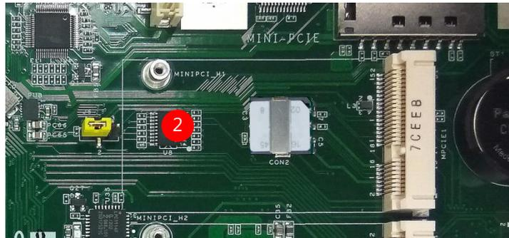
3. Follow the procedures for installing a mSATA module in the previous section to install your LTE module.
