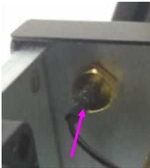
3. Use the supplied rings to secure the male connector from the front panel.
