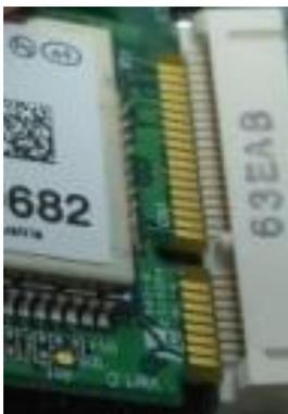
3. Press the module down and apply screws to secure it.
