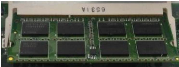
5. Insert the module into the slot at a diagonal angle and press it down until it's firmly seated by the clips at both sides.
