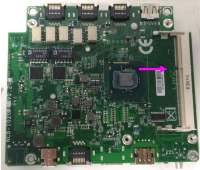
4. Align the DIMM module and make sure the notches of the module aligned with the socket keys in the slot.
