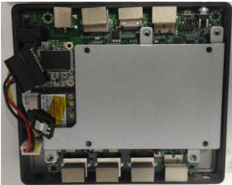
2. Make sure the screw holes are aligned and then apply screws to secure the installation between the SSD and the bracket.
