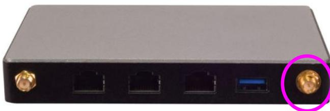
4. Tighten the rings and install the antenna. When installing the antenna, rotate it until it is tightened.
