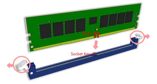
**4.** Push the module down into the slot until it is firmly seated. Press vertically on both corners of the card until it clicks into place.
