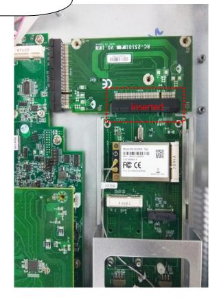
**4.** Once the expansion card is firmly seated, rotate clockwise and tighten the two lock-screws to secure the card, and then recover the system's top cover.
