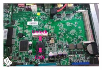
Note: To remove the SIM card, push the card outward to unlock it.
