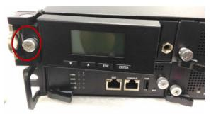
2. Open the hinge LCM and locate the HDD/SSD bays as the images shown below.
