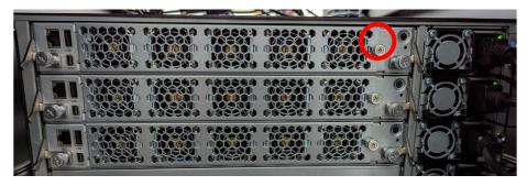
3. Hold onto the loosened captive screw and remove the bezel.
