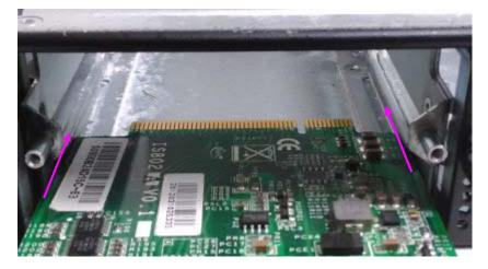
6. Apply and fasten two screws to secure the module.
