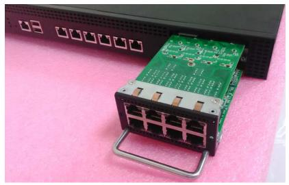
5. When sliding the module into the slot, make sure the module properly stays in the guides of the expansion space.
