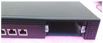
3. Orient the module in the correction direction. Make sure the LAN ports are facing you while the gold fingers are facing the expansion space.
