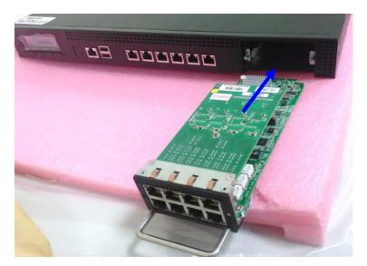
4. Insert the modules until it is firmly seated at the back of the expansion space. You should hear a "click" sound.
