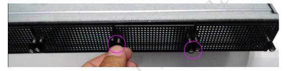
2. Remove the bezel of the module space and save it.
