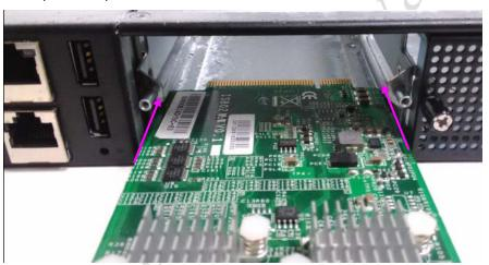
6. Rotate the captive screws until they are both secured and locked. It is strongly recommended to apply screw driver to tighten the captive screws totally.
