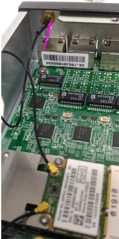
3. Use the supplied rings to secure the male connector from the front panel.
