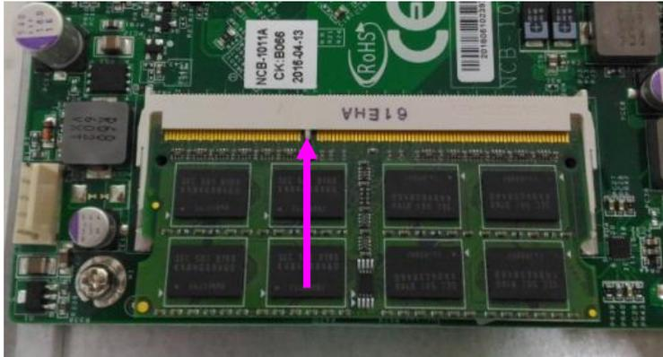
3. Insert the module into the slot in a diagonal angle and press it down until it's firmly seated by the clips at both sides.
