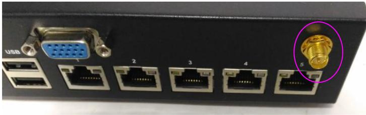
4. Tighten the rings and install the antenna. When installing the antenna, rotate it until it is tightened.
