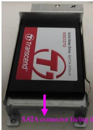
4. Turn the tray with SSD upside down and apply four screws.
