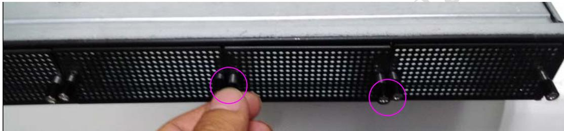
2. Remove the bezel of the module space and save it.
