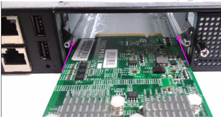
6. Rotate the captive screws until they are both secured and locked. It is strongly recommended to apply screw driver to tighten the captive screws totally.
