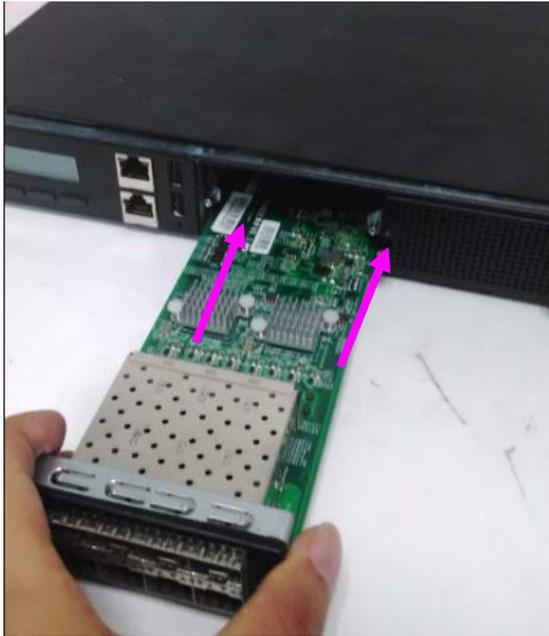
5. When sliding the module into the slot, make sure the module properly stays in the guides of the expansion space.
