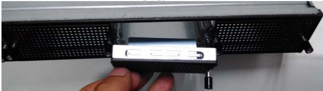
3. Position the module as shown in the image below. The PCIe gold fingers face into the module space.
