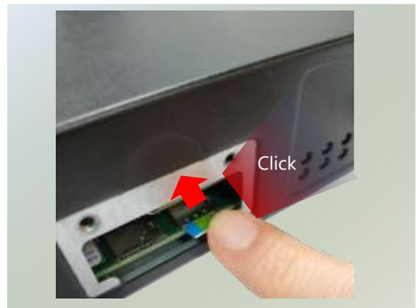
3. To remove the SIM card, use your fingertip to push it once and the card will automatically ejected.
