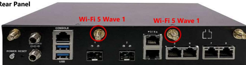
**Wi-Fi5 W2: Antenna Placement for 1x Wi-Fi 5 (802.11ac Wave 2) module**
