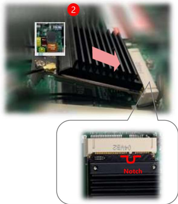
3. Secure the module with one (1) screw (included in the accessory pack).
