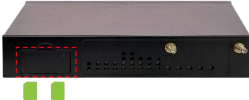
1. Locate the SIM slot cover on the front panel. Loosen the two screws that secure the SIM slot cover and remove the slot cover.
