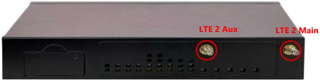
**5G: Antenna Placement for 1x 5G module**
