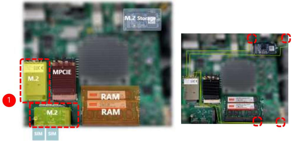
2. Align the notches of the module card with the socket keys in the slot. Tilt the end of the gold fingers down while carefully inserting the card into the slot.
