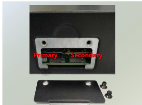
2. With the gold contacts on the SIM card facing downwards and the cut edge of the SIM card facing the left side, push the SIM card all the way in until it clicks into place.
