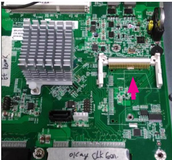
**Note:** The device has an error proof design so that the card will not be inserted if it is in the wrong orientation. You should insert the CF card with the arrow on the CompactFlash facing up and pointing toward the connector.
