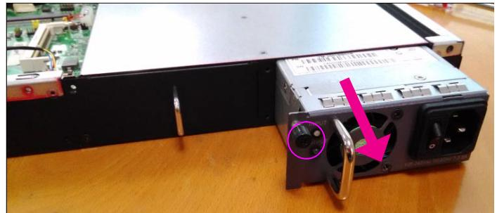
3. Once the old PSU is removed, locate the internal PSU connector and install a new PSU.
