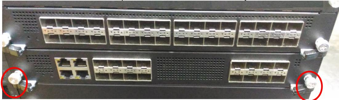
2. Pull the two locks frontwards, then extend outwards (in the same direction).
