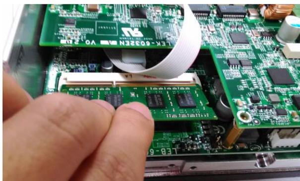
5. Press the module down until it is locked by the two clips at each side.
