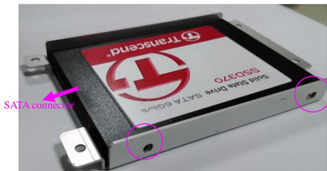
4. Place the disk drive tray back to its original place and fix it with 4 screws.
