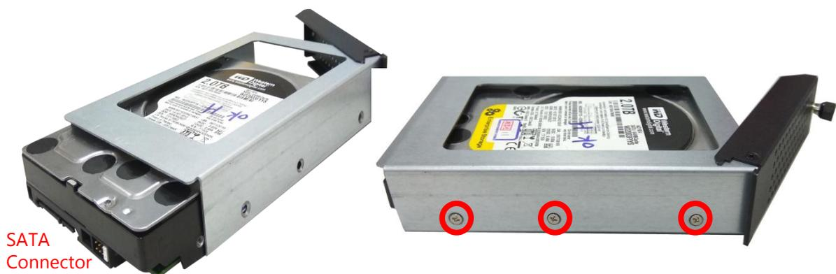
4. Insert the tray into the bay and fasten the screw that fixes the hard disk tray on the front panel.
