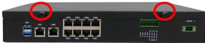
2. Pull the top cover panel open horizontally, and then lift to remove it.
