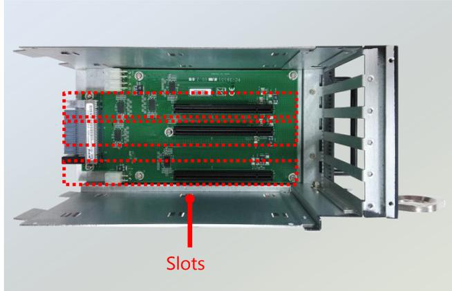
2. Vertically insert the PCIe adapter into the slot. Make sure the gold-plated connector sits well in the slot.
