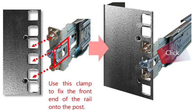
10. For the rear rack installation, slide the rail to aim and engage the bolts on the rail's rear end with the 2 available holes on the post, and the rail assembly will click into place.
