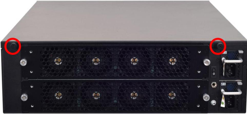
2. Pull the cover open horizontally, and then lift it up remove it.
