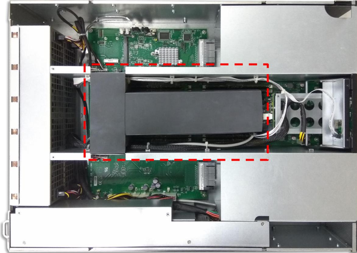
To install it after you finish servicing the components, simply place it back into the original position, and make sure the tabs on both duct sides are properly inserted into the slots shown in the picture below.
