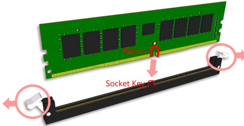
3. Push the module down into the slot until it is firmly seated. Press vertically on both corners of the card until it clicks into place.
