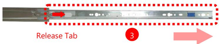
4. Remove the Rail Bracket from the Inner Channel by pushing the Release Tab on the Rail Bracket outwards while sliding it out.
