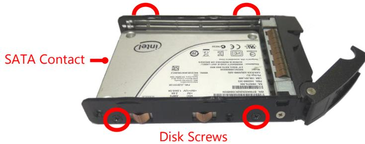
2. To install the mounted disk tray, push the tray into position in the chassis. Press on the hinge tab to close it.
