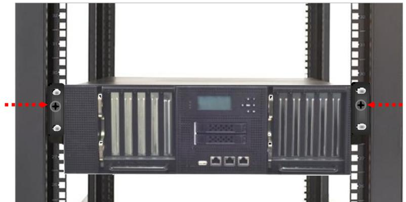
4. To remove the system from the rack, gently pull the system outwards towards you while pushing the Release Tab on both sides of the Rail Brackets.
