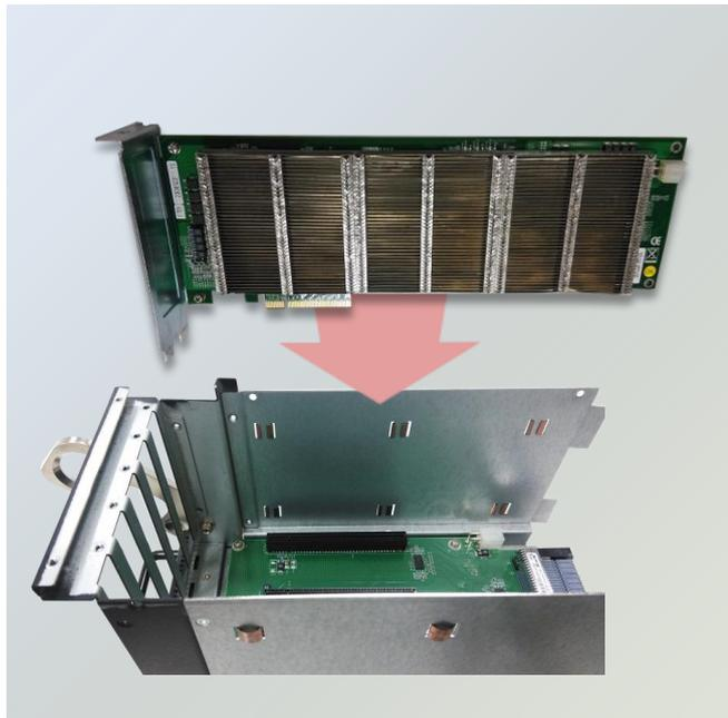
3. Fix the adapter on the riser board with screws.
