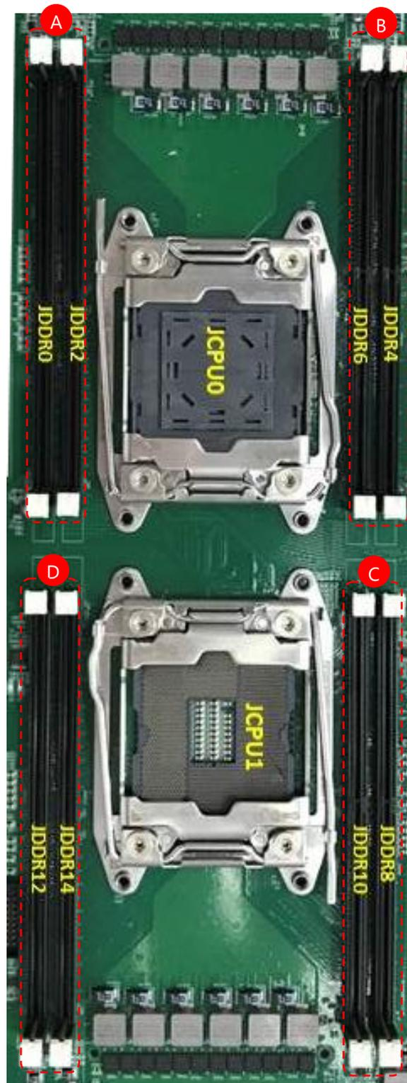
DIMM slots in Pair A and B are assigned to **CPU0**.
