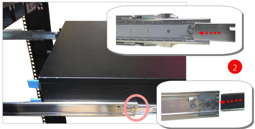
While pushing in the system, please also push and hold the Rail Lock tab on both Rail Brackets.
