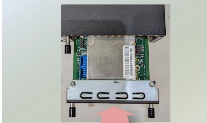
4. Once the module is firmly seated, rotate counter-clockwise and tighten the two (2) lock-screws. The NIC module has been successfully installed.
