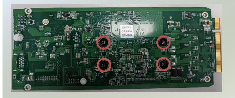
10. Turn the motherboard back around and secure the motherboard with four (4) screws.
