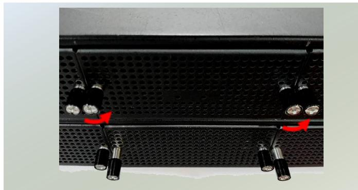
3. Remove the door and insert the module.
