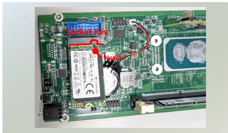
6. Insert the M.2 memory card pins at 30 degrees into the socket until it is fully seated.
