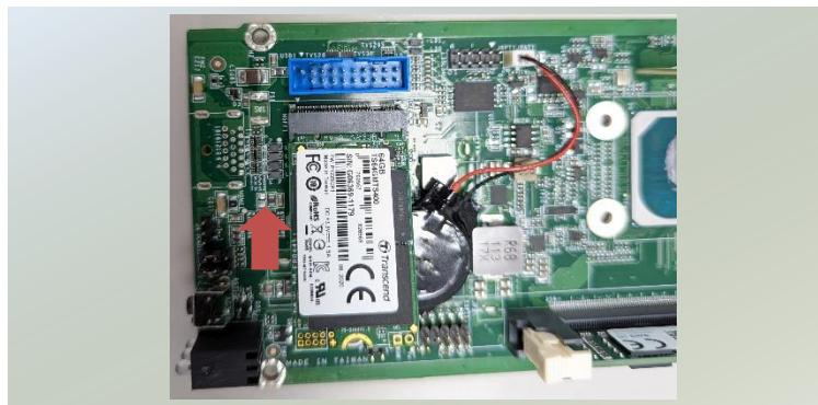
7. Push down on the module and secure it with a screw.
